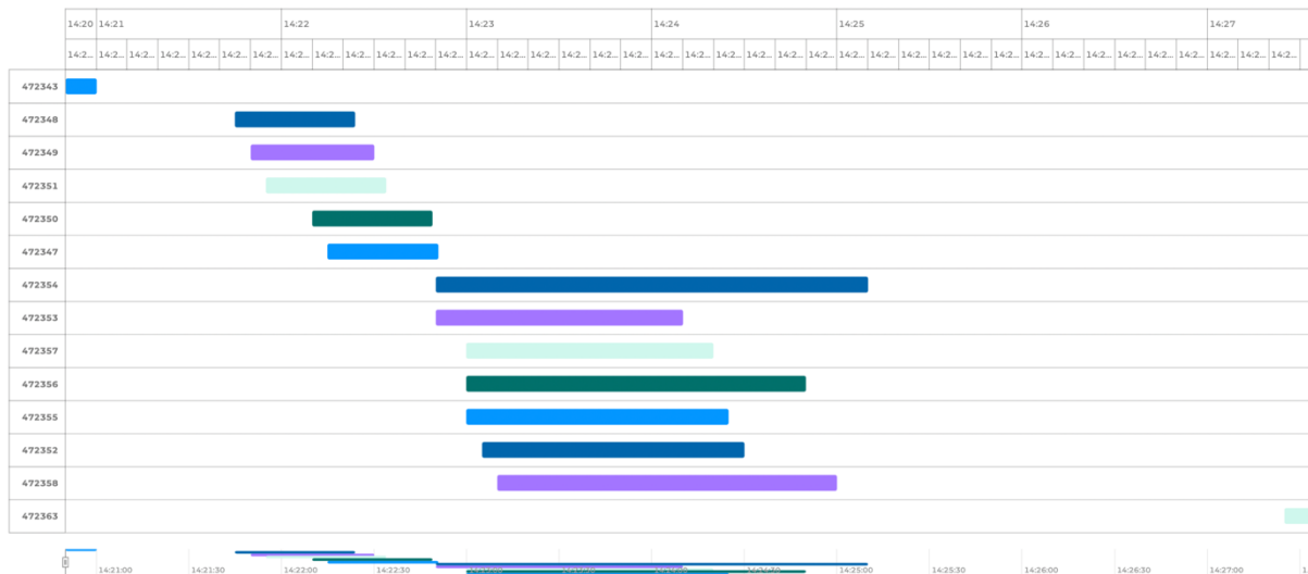
Figure 3.1: Timeline of weather forecasting benchmark workflow with five I/O simulators and seven staggered product generation jobs.
