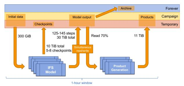
Figure 6: Weather forecasting data flow. One instance of the IFS model is run at high resolution and 51 instances are run as an ensemble at coarser resolution. Each step of the high-resolution run and each common step of the ensemble trigger one product generation run.
