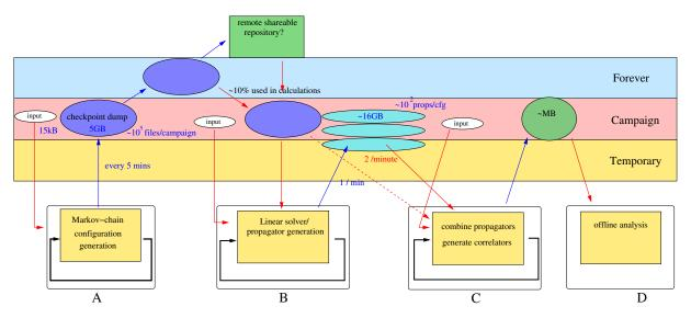
Figure 10: LQCD workflow diagram, showing data movement through the storage hierarchy for four workflow steps. step *A* is gauge configuration generation, and B - D are steps of the measurement phase. Purple ovals represent gauge configurations, cyan ovals are quark propagators, and the green oval represents hadron correlators.
