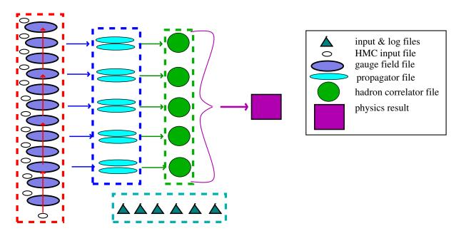
Figure 11: LQCD workflow data dependence. Red arrows represent step A HMC jobs producing gauge files (purple ovals) and restart input files (small white ovals). Step B solver jobs (blue arrows) each produce a set of propagators from a given gauge file. Step C contraction jobs (green arrows) combine propagators to produce hadron correlators (green ovals). Finally, in step D, offline analysis of the set of hadron correlators, produces a physics result (purple square).
