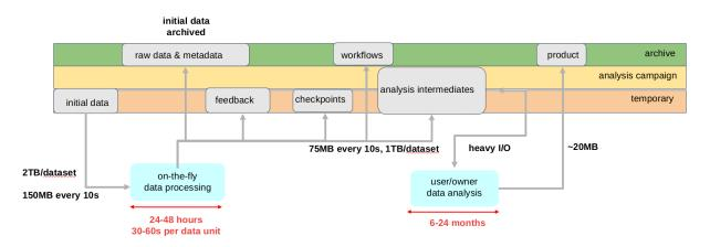
Figure 4: Electron microscopy data workflow diagram depicting the life-cycle of the cryo-EM data in the pipeline developed within the IO-SEA use case.
