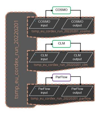
Figure 8: TSMP namespaces and their relationship to the component models.
